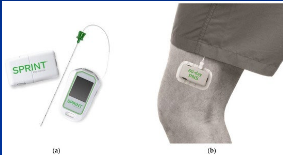
SPR Therapeutics' Sprint peripheral nerve stimulation system is constructed using a tiny 100-micron wire, about the size of a human hair.
